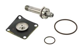
GC Valves rebuild kit, for use with S211 series DC valves ending V5CG4 and V5DG4, includes diaphragm assembly, plunger assembly, plunger tube, plunger spring, body O-ring and operator O-ring.
