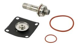
GC Valves rebuild kit, for use with S211 series AC valves ending N5EG5, includes diaphragm assembly, plunger assembly, plunger tube, plunger spring, body O-ring and operator O-ring.
