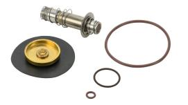
GC Valves rebuild kit, for use with S211 series AC valves ending K4EG5, includes diaphragm assembly, diaphragm spring, plunger assembly, plunger tube, plunger spring, body O-rings and operator O-ring.
