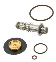
GC Valves rebuild kit, for use with S211 series AC valves ending K4DG1, includes diaphragm assembly, diaphragm spring, plunger assembly, plunger tube, plunger spring, body O-rings and operator O-ring.
