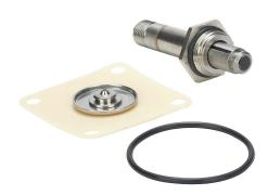
GC Valves rebuild kit, for use with NS211 series DC valves ending CG4 and DG4, includes diaphragm assembly, plunger-seat discspring assembly, plunger tube, body O-ring and operator O-ring.
