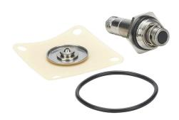
GC Valves rebuild kit, for use with NS211 series AC valves ending EG5, includes diaphragm assembly, plunger assembly, plunger tube, plunger spring, body O-ring and operator O-ring.
