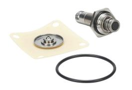
GC Valves rebuild kit, for use with NS211 series AC valves ending CG4 and DG4, includes diaphragm assembly, plunger assembly, plunger tube, plunger spring, body O-ring and operator O-ring.
