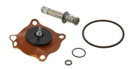
GC Valves rebuild kit, for use with S201 series AC valves ending V5FG9, includes diaphragm assembly, diaphragm spring, plunger assembly, plunger tube, plunger spring, connecting spring, body O-rings and operator O-ring.
