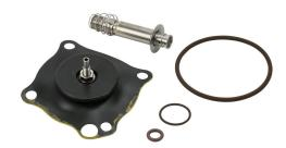
GC Valves rebuild kit, for use with S201 series DC valves ending V5FG9, includes diaphragm assembly, plunger assembly, plunger tube, plunger spring, connecting spring, body O-rings and operator O-ring.
