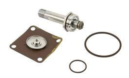
GC Valves rebuild kit, for use with S201 series AC valves ending V5EG5, includes diaphragm assembly, plunger assembly, plunger tube, plunger spring, connecting spring, body O-ring and operator O-ring.
