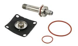
GC Valves rebuild kit, for use with S201 series DC valves ending V5CG4 and V5DG4, includes diaphragm assembly, plunger assembly, plunger tube, plunger spring, connecting spring, body O-ring and operator O-ring.
