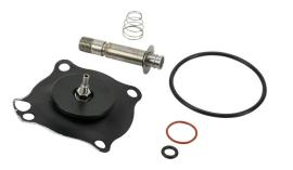
GC Valves rebuild kit, for use with S201 series DC valves ending N5FG9, includes diaphragm assembly, plunger assembly, plunger tube, plunger spring, connecting spring, body O-rings and operator O-ring.
