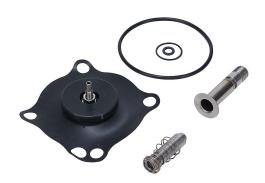
GC Valves rebuild kit, for use with NS201 series DC valves ending J2, includes diaphragm assembly, plunger assembly, plunger tube, plunger spring, plunger connecting spring, body O-rings and operator O-ring.
