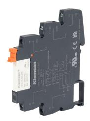
Klemsan interface relay, 35mm DIN rail mount, finger-safe, 230 VAC/VDC coil voltage, SPDT, (1) N.O., (1) N.C., 6A contact rating, screw terminal(s), LED indicator(s).
