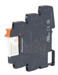
Klemsan interface relay, 35mm DIN rail mount, finger-safe, 230 VAC coil voltage, SPDT, (1) N.O., (1) N.C., 6A contact rating, screw terminal(s), LED indicator(s). Integrated leakage current suppression filter.
