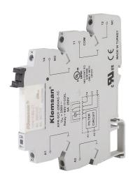
Klemsan interface relay, 35mm DIN rail mount, finger-safe, 230 VAC coil voltage, SPDT, (1) N.O., (1) N.C., 6A contact rating, screw terminal(s), LED indicator(s). Integrated leakage current suppression filter.
