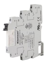
Klemsan interface relay, 35mm DIN rail mount, finger-safe, 115 VAC/VDC coil voltage, SPDT, (1) N.O., (1) N.C., 6A contact rating, screw terminal(s), LED indicator(s). Integrated leakage current suppression filter.
