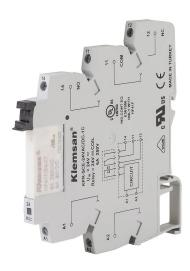
Klemsan interface relay, 35mm DIN rail mount, finger-safe, 24 VAC/VDC coil voltage, SPDT, (1) N.O., (1) N.C., 6A contact rating, screw terminal(s), LED indicator(s).
