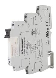
Klemsan interface relay, 35mm DIN rail mount, finger-safe, 230 VAC/VDC coil voltage, SPDT, (1) N.O., (1) N.C., 6A contact rating, screw terminal(s), LED indicator(s).
