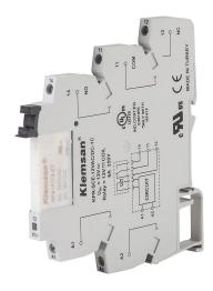
Klemsan interface relay, 35mm DIN rail mount, finger-safe, 12 VAC/VDC coil voltage, SPDT, (1) N.O., (1) N.C., 6A contact rating, screw terminal(s), LED indicator(s).
