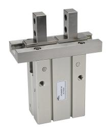
NITRA pneumatic gripper, parallel, single acting, N.C., 40mm bore, 30mm stroke, side mount grip, anodized aluminum body, M5 x 0.8 female ISO port(s).
