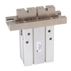
NITRA pneumatic gripper, parallel, single acting, N.C., 40mm bore, 30mm stroke, end mount grip, anodized aluminum body, M5 x 0.8 threaded port(s).
