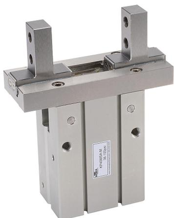
NITRA pneumatic gripper, parallel, single acting, N.O., 40mm bore, 30mm stroke, side mount grip, anodized aluminum body, M5 x 0.8 female ISO port(s).
