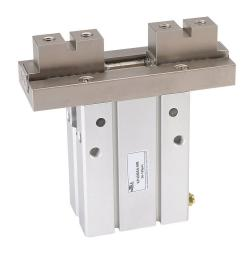
NITRA pneumatic gripper, parallel, single acting, N.O., 40mm bore, 30mm stroke, end mount grip, anodized aluminum body, M5 x 0.8 female ISO port(s).
