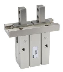
NITRA pneumatic gripper, parallel, double acting, 40mm bore, 30mm stroke, side mount grip, anodized aluminum body, M5 x 0.8 threaded port(s).
