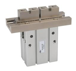
NITRA pneumatic gripper, parallel, double acting, 40mm bore, 30mm stroke, end mount grip, anodized aluminum body, M5  $\times$  0.8 female ISO port(s).
