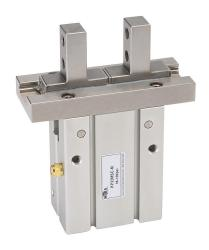
NITRA pneumatic gripper, parallel, single acting, N.C., 32mm bore, 22mm stroke, side mount grip, anodized aluminum body, M5 x 0.8 threaded port(s).
