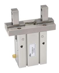
NITRA pneumatic gripper, parallel, single acting, N.O., 32mm bore, 22mm stroke, side mount grip, anodized aluminum body, M5 x 0.8 female ISO port(s).
