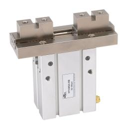
NITRA pneumatic gripper, parallel, single acting, N.O., 32mm bore, 22mm stroke, end mount grip, anodized aluminum body, M5 x 0.8 female ISO port(s).
