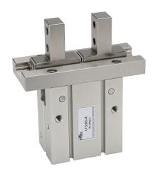
NITRA pneumatic gripper, parallel, double acting, 32mm bore, 22mm stroke, side mount grip, anodized aluminum body, M5  $\times$  0.8 female ISO port(s).
