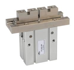
NITRA pneumatic gripper, parallel, double acting, 32mm bore, 22mm stroke, end mount grip, anodized aluminum body, M5 x 0.8 threaded port(s).
