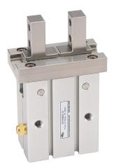
NITRA pneumatic gripper, parallel, single acting, N.C., 25mm bore, 14mm stroke, side mount grip, anodized aluminum body, M5 x 0.8 female ISO port(s).
