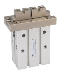
NITRA pneumatic gripper, parallel, single acting, N.C., 25mm bore, 14mm stroke, end mount grip, anodized aluminum body, M5 x 0.8 female ISO port(s).
