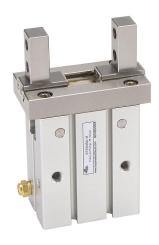
NITRA pneumatic gripper, parallel, single acting, N.O., 25mm bore, 14mm stroke, side mount grip, anodized aluminum body, M5 x 0.8 threaded port(s).
