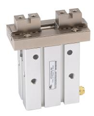
NITRA pneumatic gripper, parallel, single acting, N.O., 25mm bore, 14mm stroke, end mount grip, anodized aluminum body, M5 x 0.8 female ISO port(s).
