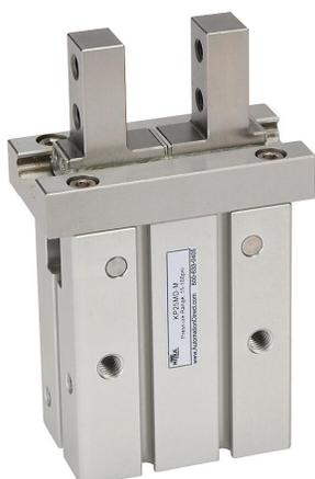
NITRA pneumatic gripper, parallel, double acting, 25mm bore, 14mm stroke, side mount grip, anodized aluminum body, M5 x 0.8 female ISO port(s).
