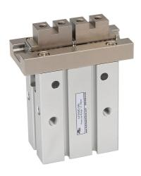
NITRA pneumatic gripper, parallel, double acting, 25mm bore, 14mm stroke, end mount grip, anodized aluminum body, M5  $\times$  0.8 female ISO port(s).
