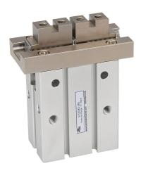
NITRA pneumatic gripper, parallel, double acting, 25mm bore, 14mm stroke, end mount grip, anodized aluminum body, M5  $\times$  0.8 threaded port(s).
