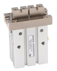
NITRA pneumatic gripper, parallel, single acting, N.C., 20mm bore, 10mm stroke, end mount grip, anodized aluminum body, M5 x 0.8 female ISO port(s).
