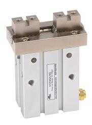
NITRA pneumatic gripper, parallel, single acting, N.O., 20mm bore, 10mm stroke, end mount grip, anodized aluminum body, M5 x 0.8 threaded port(s).
