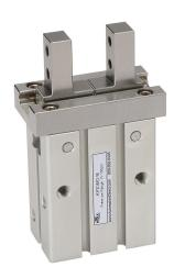
NITRA pneumatic gripper, parallel, double acting, 20mm bore, 10mm stroke, side mount grip, anodized aluminum body, M5  $\times$  0.8 threaded port(s).
