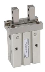
NITRA pneumatic gripper, parallel, double acting, 20mm bore, 10mm stroke, side mount grip, anodized aluminum body, M5 x 0.8 female ISO port(s).
