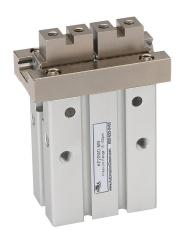
NITRA pneumatic gripper, parallel, double acting, 20mm bore, 10mm stroke, end mount grip, anodized aluminum body, M5  $\times$  0.8 female ISO port(s).
