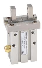
NITRA pneumatic gripper, parallel, single acting, N.C., 16mm bore, 6mm stroke, side mount grip, anodized aluminum body, M5  $\times$  0.8 threaded port(s).
