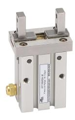
NITRA pneumatic gripper, parallel, single acting, N.O., 16mm bore, 6mm stroke, side mount grip, anodized aluminum body, M5  $\times$  0.8 female ISO port(s).
