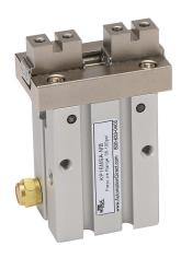
NITRA pneumatic gripper, parallel, single acting, N.O., 16mm bore, 6mm stroke, end mount grip, anodized aluminum body, M5 x 0.8 female ISO port(s).
