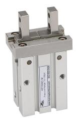
NITRA pneumatic gripper, parallel, double acting, 16mm bore, 6mm stroke, side mount grip, anodized aluminum body, M5 x 0.8 female ISO port(s).
