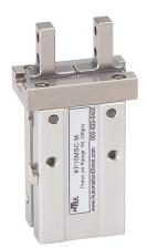
NITRA pneumatic gripper, parallel, single acting, N.C., 10mm bore, 4mm stroke, side mount grip, anodized aluminum body, M3 x 0.5 female ISO port(s).
