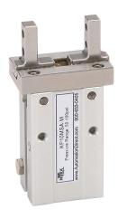
NITRA pneumatic gripper, parallel, single acting, N.O., 10mm bore, 4mm stroke, side mount grip, anodized aluminum body, M3  $\times$  0.5 female ISO port(s).
