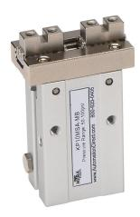
NITRA pneumatic gripper, parallel, single acting, N.O., 10mm bore, 4mm stroke, end mount grip, anodized aluminum body, M3  $\times$  0.5 threaded port(s).
