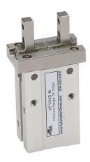
NITRA pneumatic gripper, parallel, double acting, 10mm bore, 4mm stroke, side mount grip, anodized aluminum body, M3  $\times$  0.5 threaded port(s).
