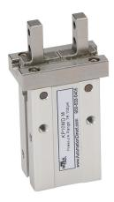
NITRA pneumatic gripper, parallel, double acting, 10mm bore, 4mm stroke, side mount grip, anodized aluminum body, M3 x 0.5 female ISO port(s).
