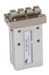
NITRA pneumatic gripper, parallel, double acting, 10mm bore, 4mm stroke, end mount grip, anodized aluminum body, M3 x 0.5 female ISO port(s).
